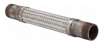
This "flexible metal hose" is ideal to make flexible connections to tanks, pumps, or wherever some piping flexibility is required. They can withstand heat, cold, and high pressures. These are available in sizes from ½" to 6" and even larger.
