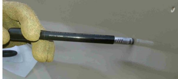
Above is an example of mil thickness testing being completed on a powder coated tank.
